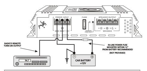
**IMPORTANT!** Before making any connections, disconnect the car's battery until the installation is completed to avoid possible damage to the electrical system.
